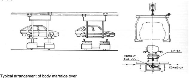
Fig. 8.3 Body position for Docking of Power-train
