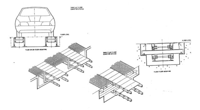
Fig. 8.10 Single Slat or Two Slat Conveyor
