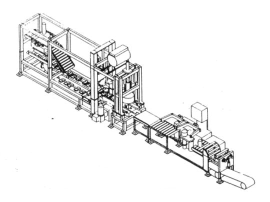
Fig. 8.4 A Tyre- Wheel Assembly System
