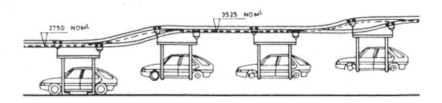
Fig. 8.5 Bodies on Tyres to Final Assembly Conveyor
