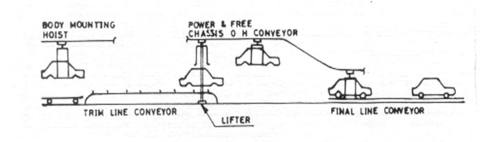
Fig. 8.2 Transfer of Car body from Trim line
