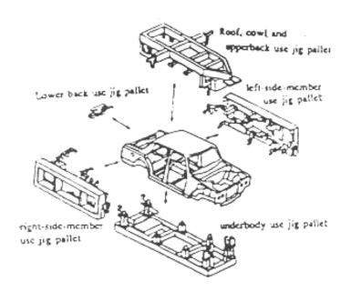
Fig. 6.13 Different Jig Pallets for Major Subassemblies
