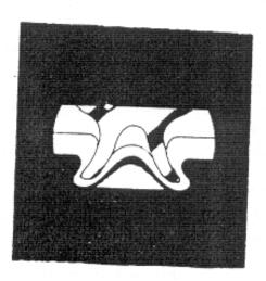
Fig. 6.19 A Self Piercing Rivet
