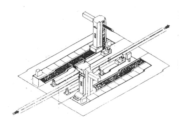
Fig. 6.21 A Robotised Cell for Body Inspection
