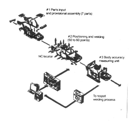
Fig. 6.14 Stages of Nissan's Intelligent Body Assembly System
