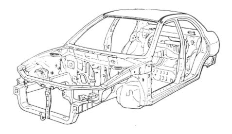
Fig. 6.2 A Typical Body Shell Construction
