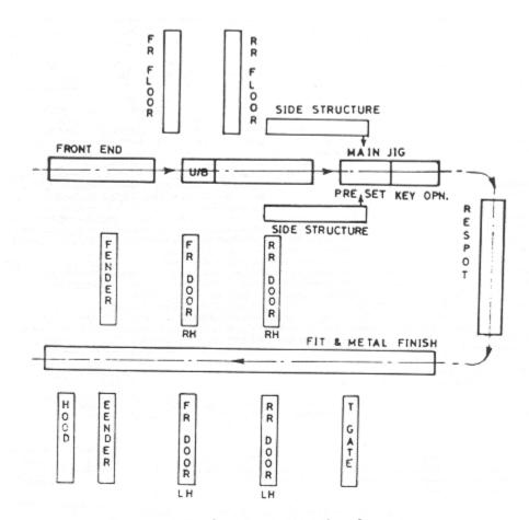
Fig. 6.1 A Typical Body Welding Shop Layout
