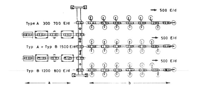
Fig. 6.5 Model Specific Tacking and Flexible Spot Welding Lines
