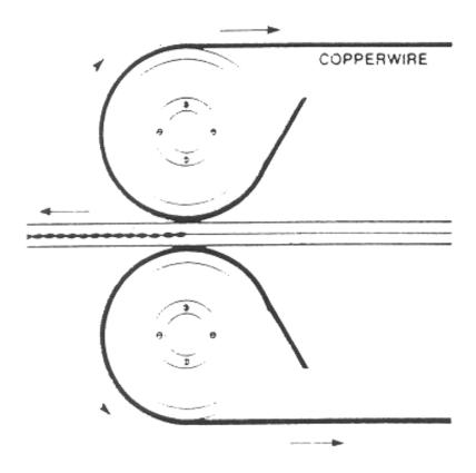
Fig. 6.17. An Improved Seam Welding for Coated Steel
