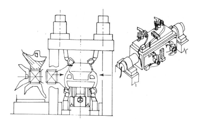
Fig. 6.7 An Improved Version of Body Framing Station
