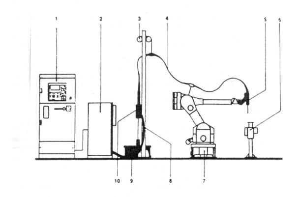
Fig. 6.16 An Arc Welding Robot
