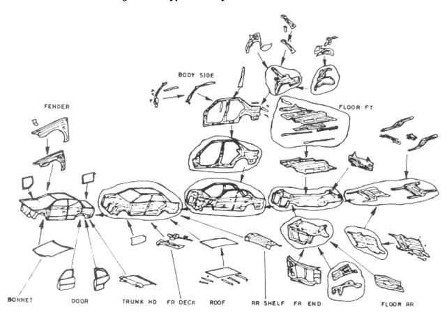
Fig. 6.3 Sequences of Sub-Assemblies and Main Body Welding
