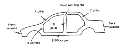
Fig. 6.18 Possible Laser Welding Areas of Autobody
